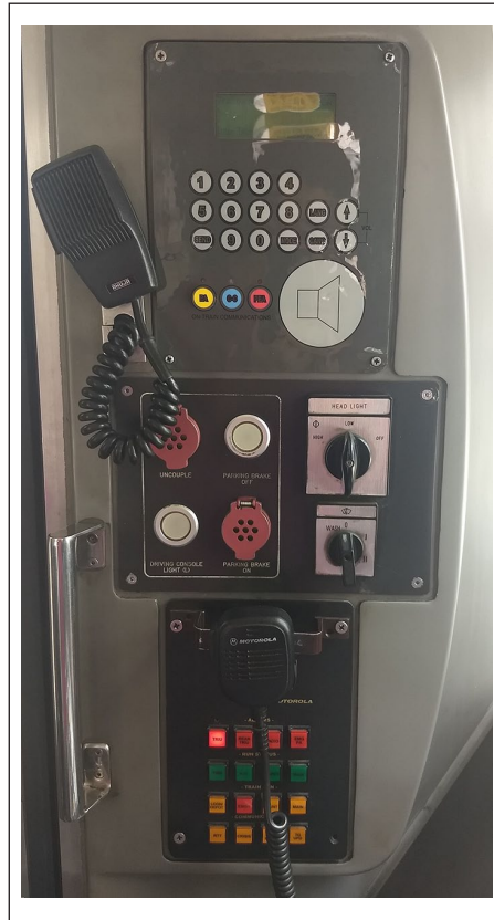
Figure 3. The in-train PA communication panel in the driver's cabin.
